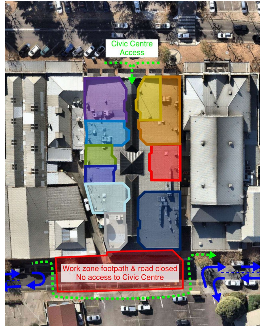
Figure 2 - Pedestrian Routes During Washington Street Crane Lift
